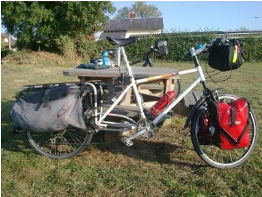
The term 'longtail' has only been applied to the bicycle since the arrival of the **Xtracycle** (pic left). As you can see, a longtail is basically a long bike, designed that way to carry extra cargo (often as much as 100kg).
