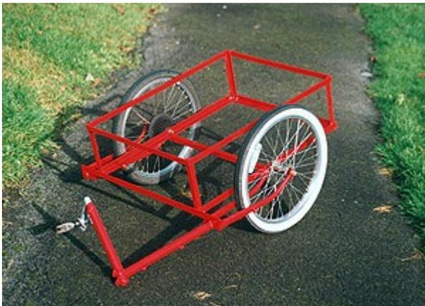
If cash is tight, you might want to consider building your own trailer. The charity Re-cycle ([www.re-cycle.org](http://www.re-cycle.org)) offers plans on how to construct a trailer from old bike parts (pictured left) which can be bolted together rather than welded. The instructions are here>>
