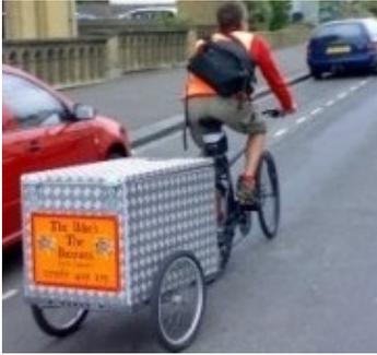
A heavy duty trailer made from steel with quality cartridge wheel bearings, designed and built by Pashley in England to carry a euro crate. The Euro comes as a flatbed with optional plastic box. Alternatively you can add your own box to suit your needs.
